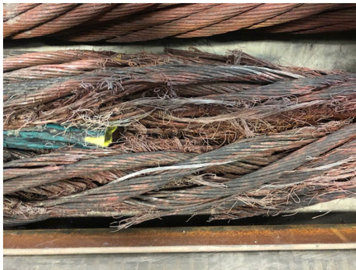
Figure 4. Example of poor copper conductor bundling and an undersized core hose. Significant wire breakage and core hose abrasion is evident.
