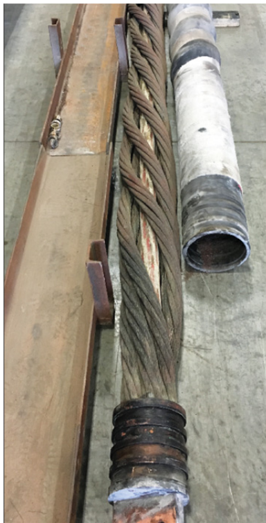
Figure 7. Example of undersized core hose permitting greater internal movement of wire conductors during electrical cycling, potentially resulting in excessive chaff and friction wear.
