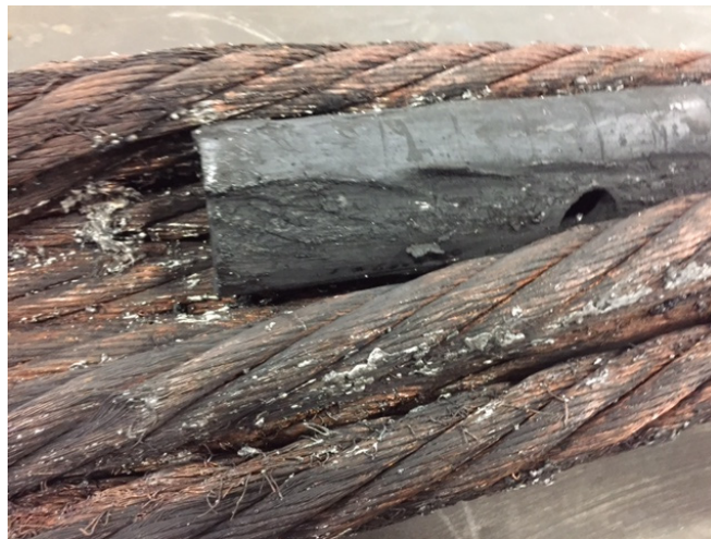
Figure 9. Example of catastrophic lack of coolant flow within power cable. Resulting heat exceeded melting point of solder. Perforated core hose is burned.
