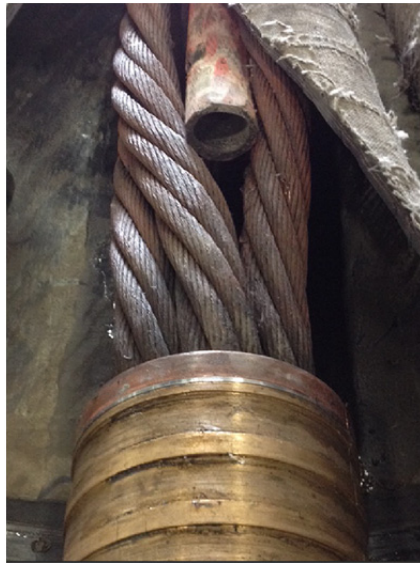
Figure 8. Example of weak low-durometer core hose with perforations, and no end plugs compounding inefficient flow of coolant to the wire conductor bundle.
