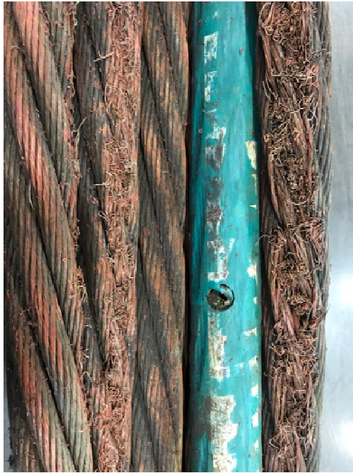
Figure 6. Example of poor copper conductor bundling and a perforated, undersized core hose. Significant wire breakage and core hose abrasion is evident.
