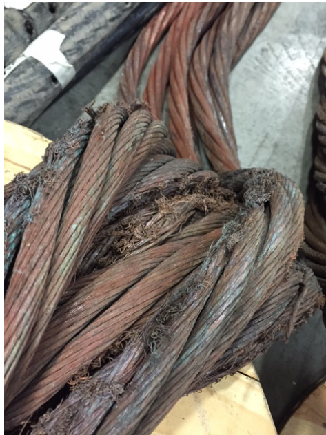
Figure 3. Example of broken conductor bundle caused by lack of core in original cable assembly.
