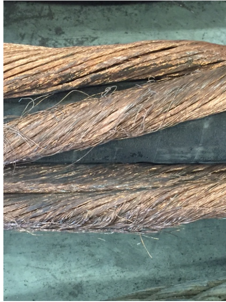
Figure 2. Example of normal wear and tear on copper conductor wire.
