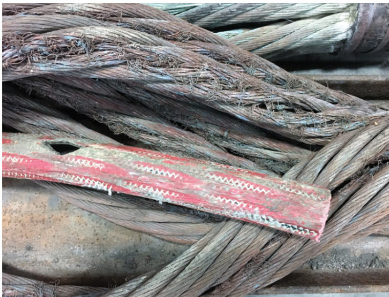
Figure 5. Example of poor copper conductor bundling and a perforated, undersized core hose. Significant wire breakage and core hose abrasion is evident.
