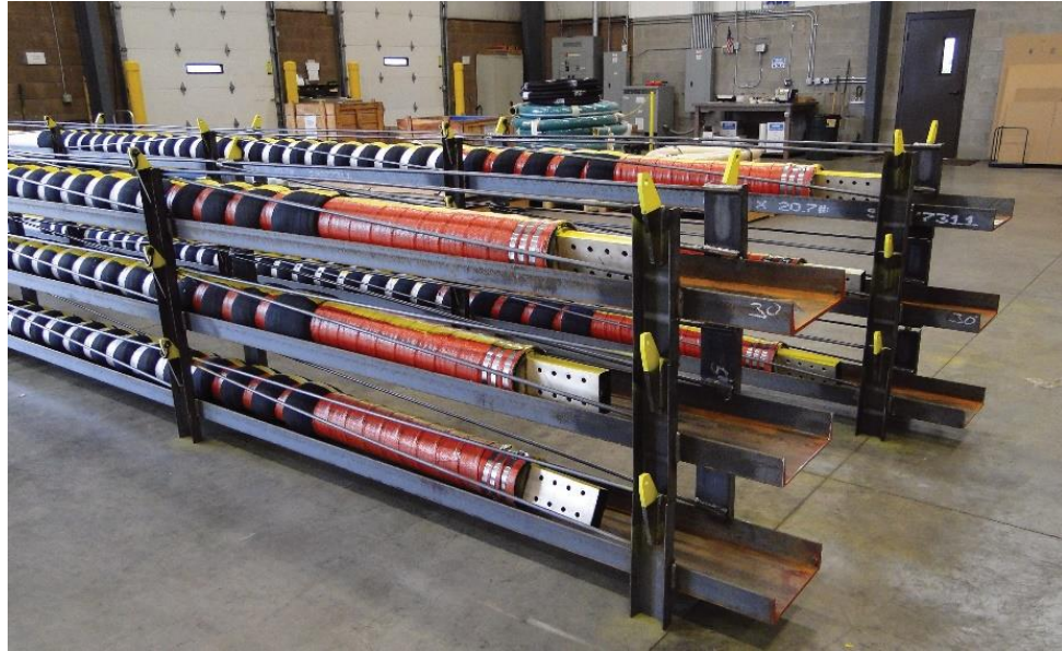
Figure 3. Newly manufactured spare cables stacked in trays for safe, portable and flat storage.
