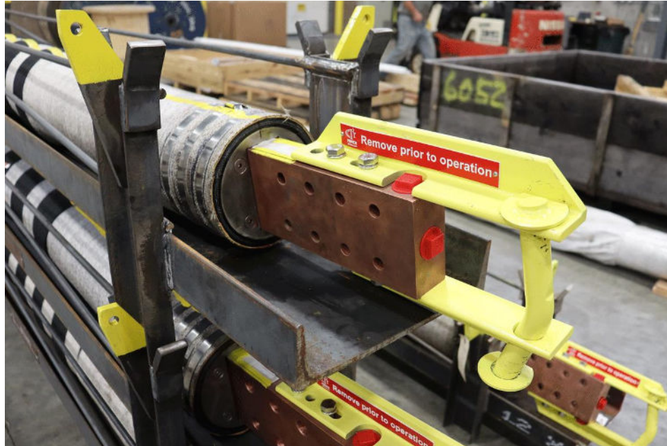
Figure 4. Newly manufactured spare EAF cables stacked in trays and fitted with custom handles for lifting and/or hanging.
