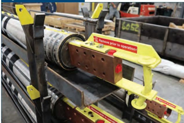
Newly manufactured spare EAF cables stacked in trays and fitted with custom handles for lifting and/or hanging.
